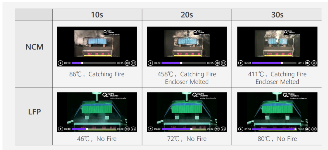
Figure 4 Safety Test Comparison Between LFP and NCM (Puncture Test) [11]
