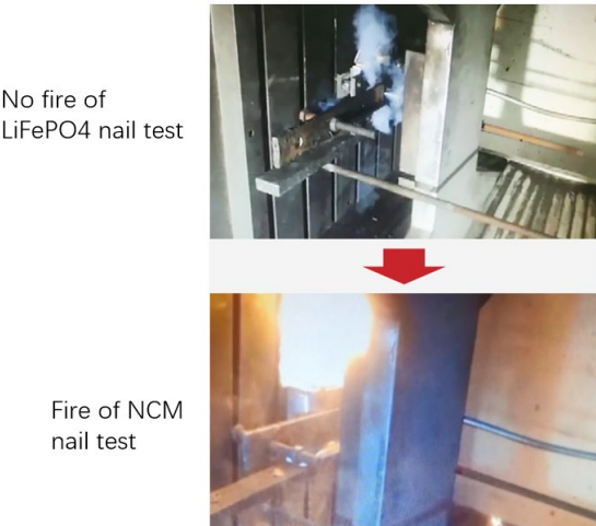
Figure 11 Nail Test of NCM and LFP
