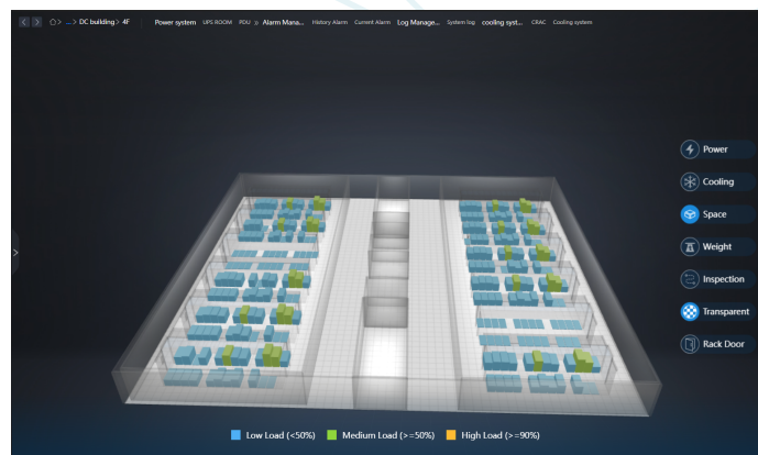
Figure 3.22. Identifying Local Hotspots in the Equipment Room by Temperature Map
