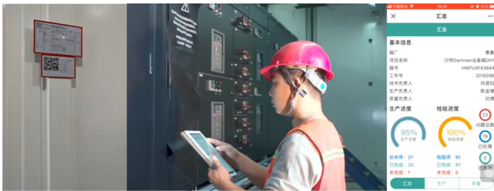
Figure 5-33 One code for one pre-fab. module, digital control for module prefabrication
