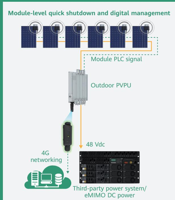
Figure 4-8 Module-level quick shutdown and digital management
