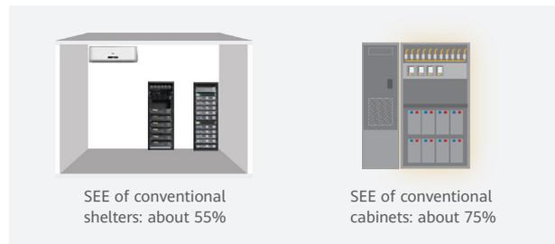
Figure 2-2 Energy efficiency of a conventional shelter and cabinet site
