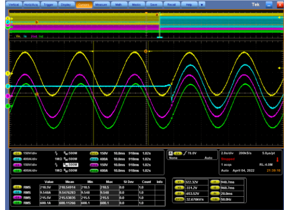
Figure 36 Recovery at normal voltage (220 V)
