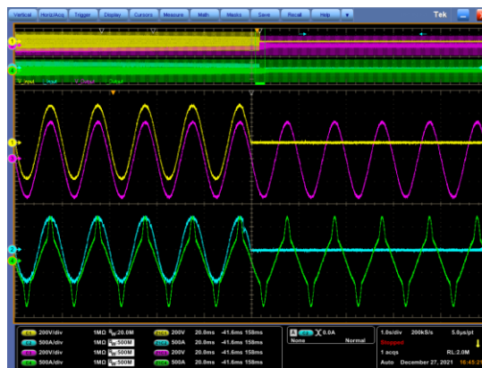
Figure 44 Yellow: bypass input voltage; blue: bypass input current; purple: system output voltage; green: system output current
