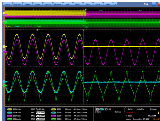
Figure 36 Yellow: bypass input voltage; blue: bypass input current; purple: system output voltage; green: system output current
