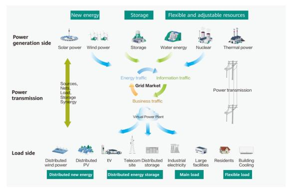
Balanced power system with energy synergy
