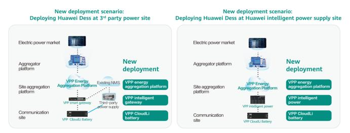
New Lithium Battery Deployment in Huawei DESS solution
